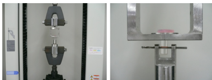
Fig. 2 Assembly for tensile bond strength testing
