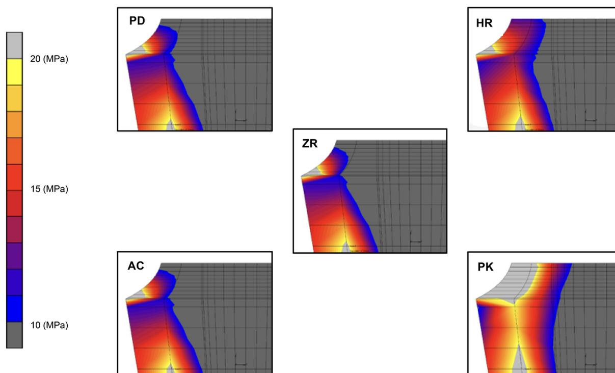
**Fig. 6** The stress distribution within the cervical area of the dentin (frontal plane)
