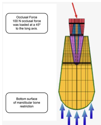
**Fig. 2** Three-dimensional occlusal force with bottom surface of mandibular restriction
