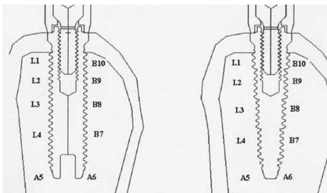
**Fig. 5.** Interface between the implant and trabecular bone along path sections L1 to B10, of each step section of stepped screw implant and corresponding section of cylindrical screw implant.
