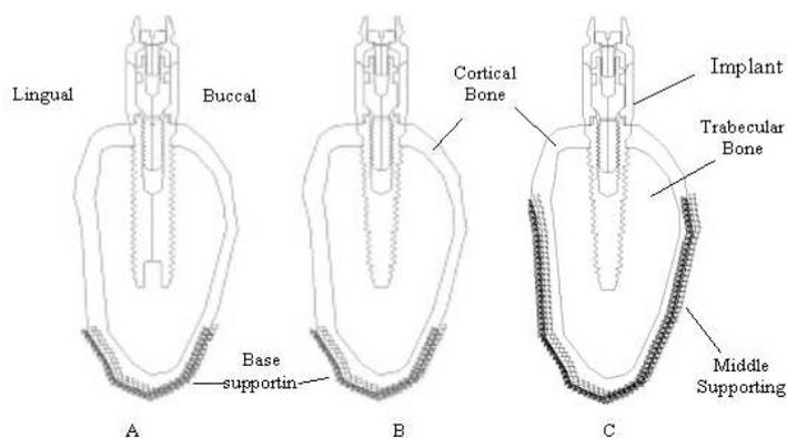
Fig. 1. Different bone-implant systems and boundary conditions.
