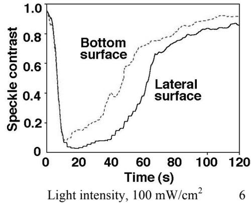
**Figs. 5, 6.** Speckle-contrast measurements of the lateral surfaces and underside as a function of time (mold diameter, 4mm; mold height, 6mm).
