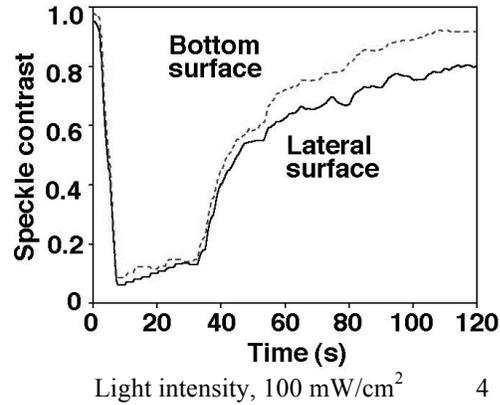
**Figs. 3, 4.** Speckle-contrast measurements of the lateral surfaces and underside as a function of time (mold diameter, 4 mm; mold height, 4mm).
