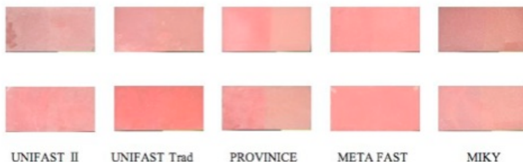
Fig. 3. Specimens after being exposed to xenon light. Upper, mixing technique; Lower, brush-on technique
