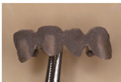
Fig. 16. Air-abrasion with alumina
