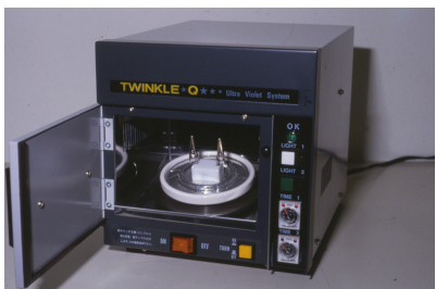
Fig. 13. Polymerization with a UV-unit
