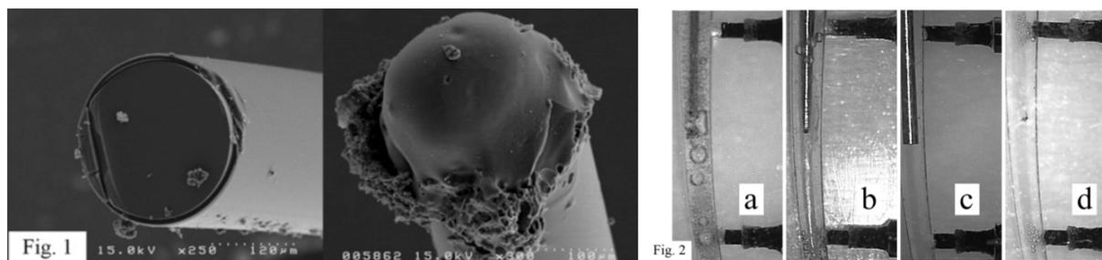
**Fig. 1** Scanning electron microscope images of the clear tip (a cylindrical fiber tip; left) and the TOP tip (right)
