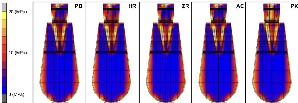
Fig. 4 The stress distribution (frontal plane)
