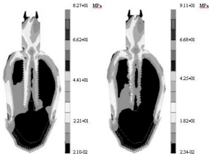
**Fig. 3.** Stress distributions under an oblique load of 141 N with normal cortical bone (left) cylindrical screw implant, and (right) stepped screw implant.
