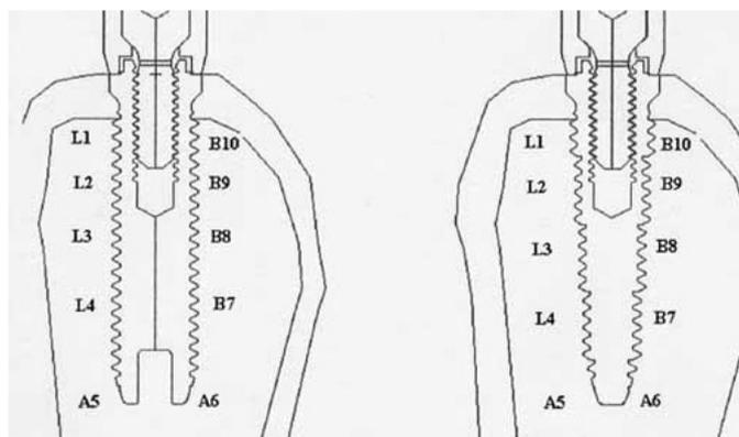
**Fig. 5.** Interface between the implant and trabecular bone along path sections L1 to B10, of each step section of stepped screw implant and corresponding section of cylindrical screw implant.
