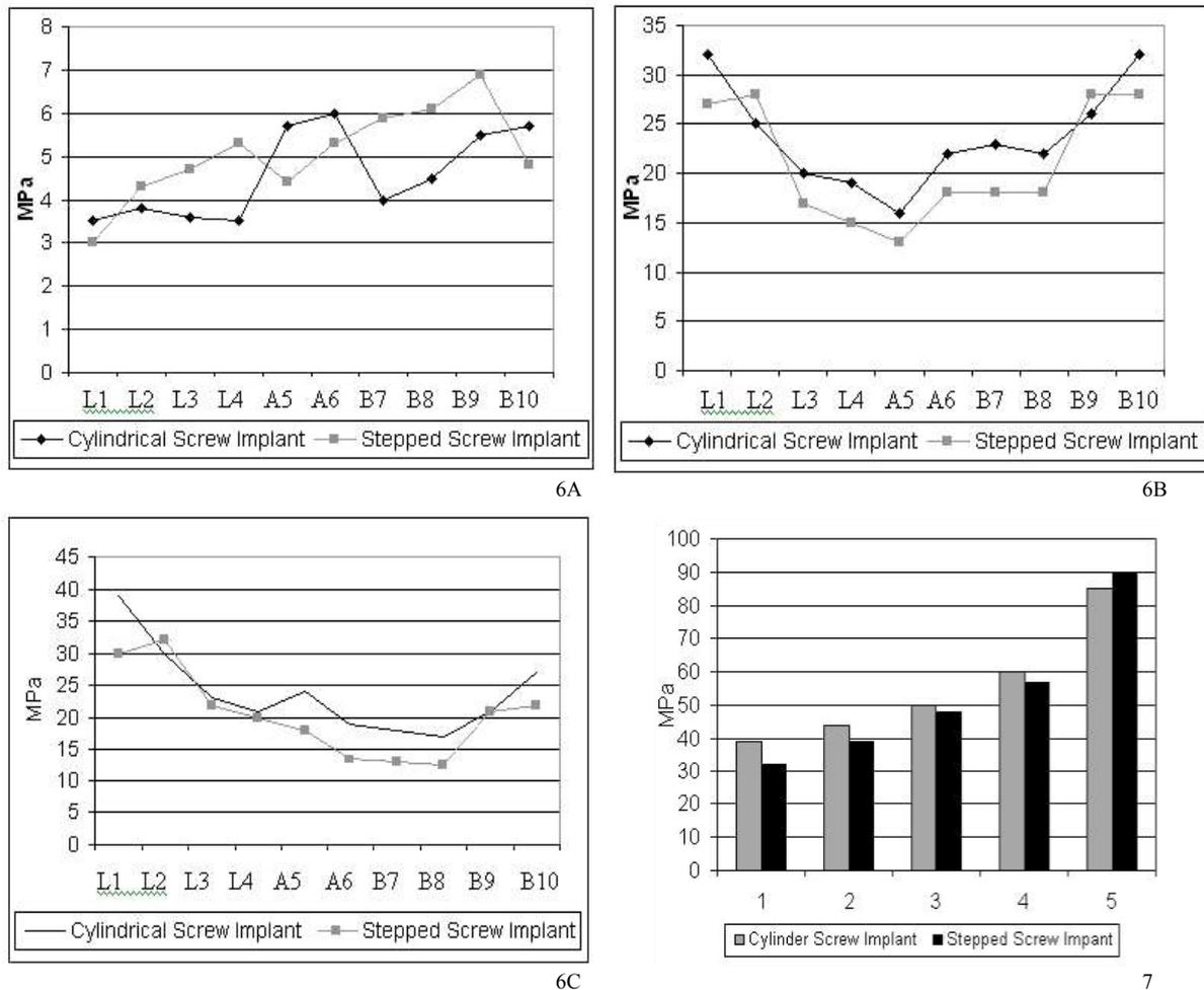
**Fig. 6.** Maximum von Mises stress at the interface along path L1 to B10 between implant and trabecular bone under A, vertical load of 100 N, B, horizontal load of 100 N, and C, oblique load of 141 N at 45 degrees inclination (L: Lingual; A: Apex; B: Buccal).
