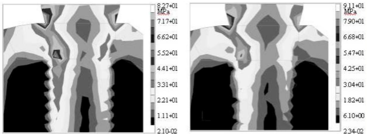
**Fig. 4.** Stress distribution of cylindrical screw implant (left) and of stepped screw implant (right) under oblique load of 141 N with condition 1 (cortical bone of E=13,400 MPa and P=0.30).
