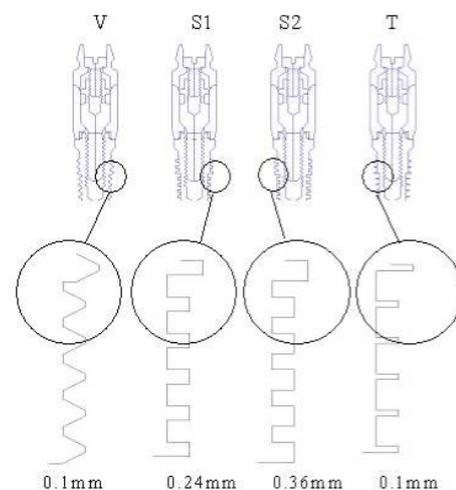
Fig. 2. Four different stepped screw implants (left) and thread configurations (right).
