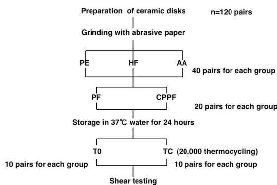
Fig. 1. Procedures for specimen preparation.
