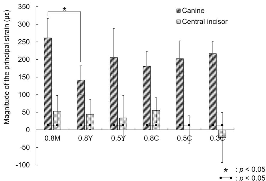
**Fig. 4** Comparison of magnitude of the principal strains for six kinds of frameworks
