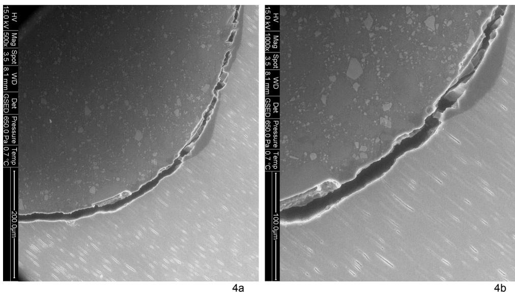
**Fig. 4** Environmental SEM observations of cavity wall-resin gap formation in a tooth restored with Clearfil Photo Bright 4a (500×), 4b (1,000×)
