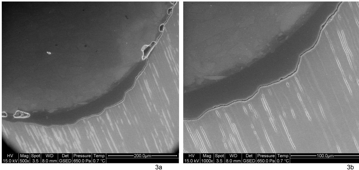
**Fig. 3** Environmental SEM observations of cavity wall-resin gap formation in a tooth restored with Palfique Estelite 3a (500×), 3b (1,000×)
