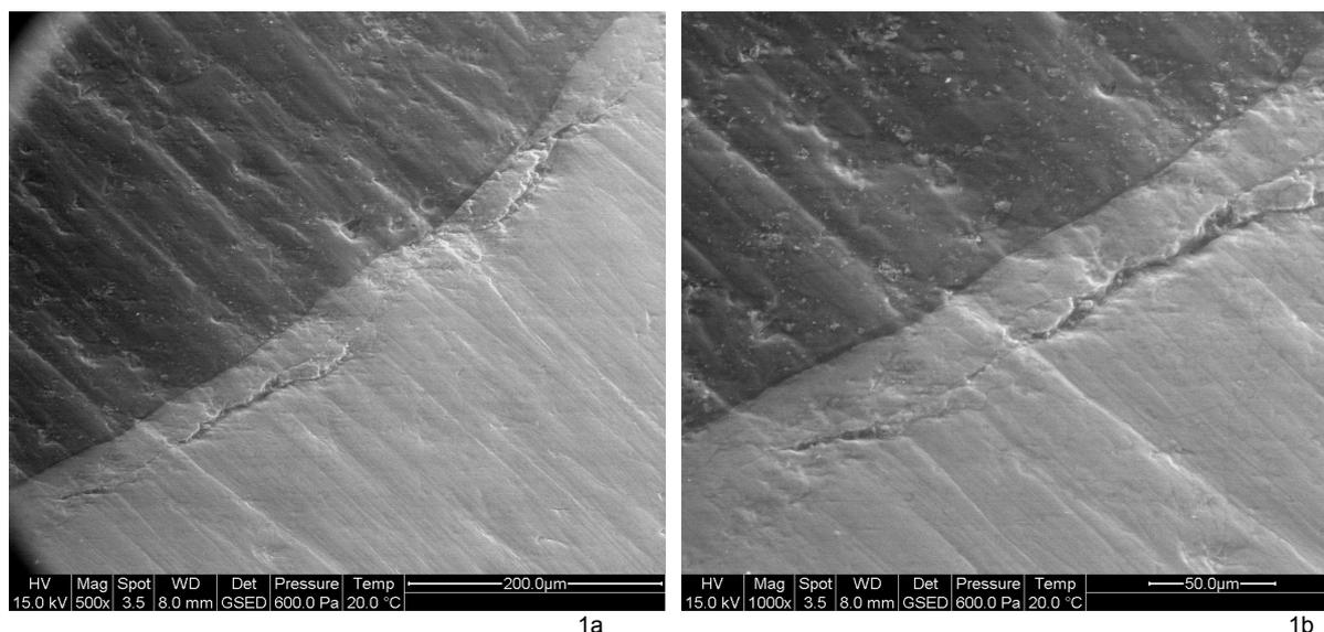
**Fig. 1** Environmental SEM observation of enamel cracks on the margins around Palfique Estelite resin composite restorations 1a (500×), 1b (1,000×)
